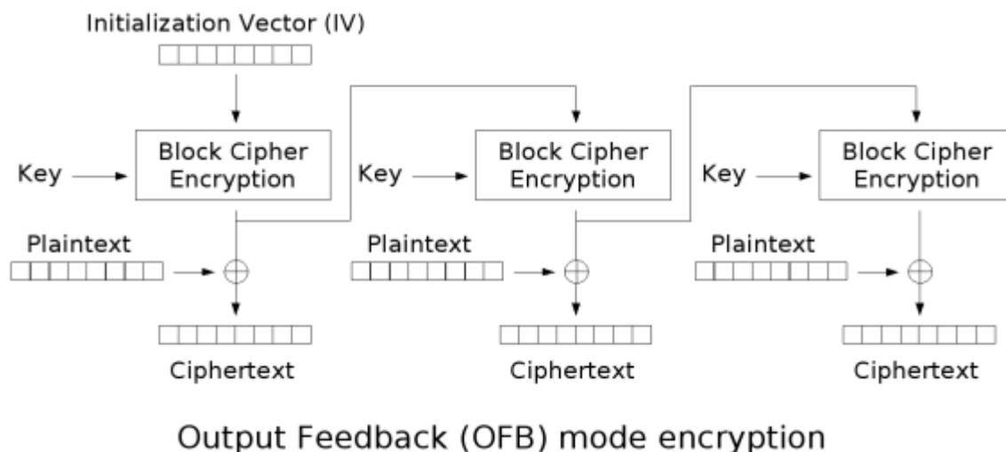
*In that mode we use also an initialization vector. The output of the block cipher encryption is XOR'd with the plaintext. In addition the output of the block cipher encryption is used as key for the next block, so that there a continuous stream of encrypted blocks arises. The bit stream is pseudo randomly because it depends on the block encryption, key and initialization vector.*
