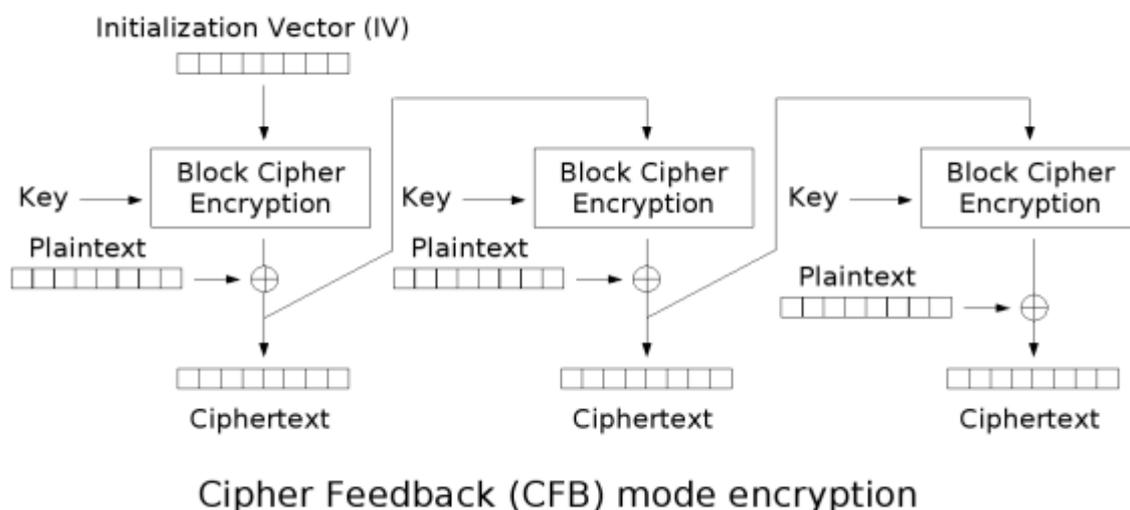
*Cipher Feedback is very similar to OFB. The difference is that the key for the next block is the ciphertext of the previous block.*
